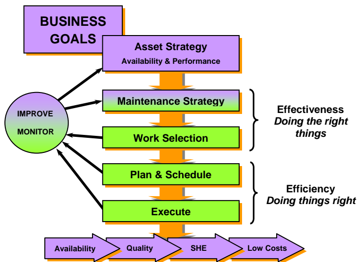
Figure 1 Rational maintenance strategy and actions cascade directly from the enterprise's business goals
